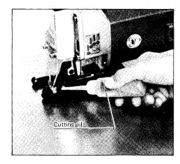
The underside of the workpiece can be greased instead of using a coolant.
